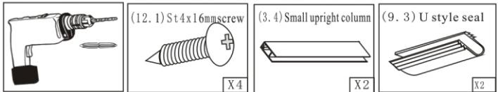
Fit U rubber seal to glass the other side, then use hammer to make the small aluminum panel(3.4) cover the glass. Then, fix the aluminum panel by screw(12.1)
