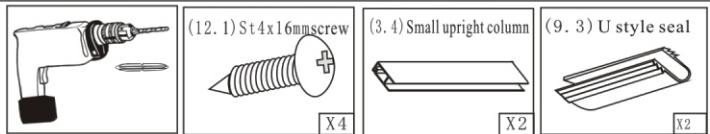
Fit U rubber seal to glass the other side, then use hammer to make the small aluminum panel(3.4) cover the glass. Then, fix the aluminum panel by screw(12.1)
