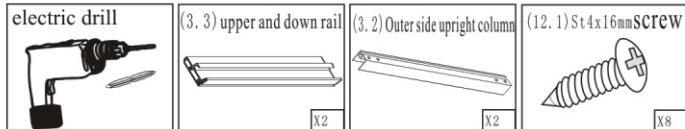
Installing the glass room frame. Take out 2 upright aluminum alloy columns and the top and bottom rails from 1/4 package. Connect them with the screws (12.1). Then put the finished frame on the tub as the “up” label at the top.
