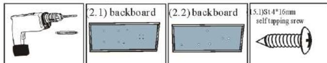
3.) Connect the aluminum panel and 2 pieces of back board glassby screws.
