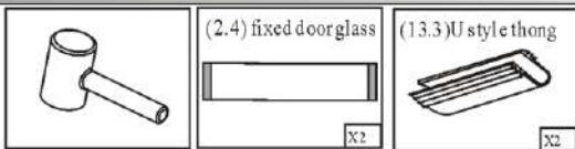
Fit the fixed glass into the frame, after fitting the rubber seal into glass one side, and then knock the glass carefully by hammer.
